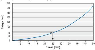
Type TR95-50H Force-Stroke Characteristic (dynamic) (with impact velocity over 0.5 m/s)
