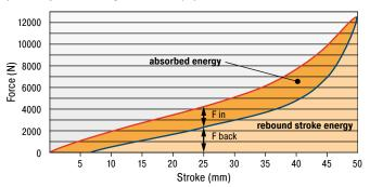
With the aid of the characteristic curves above you can estimate the proportion of the total energy that will be absorbed. Example: With impact energy of 50 Nm the Energy-Stroke diagram shows that a stroke of about 25 mm is needed. On the Force-Stroke diagram you can estimate the proportion of absorbed energy to rebound energy at this stroke length. **Dynamic (v > 0.5 \text{ m/s}) and static (v \le 0.5 \text{ m/s}) characteristics of all types are available on request.**
