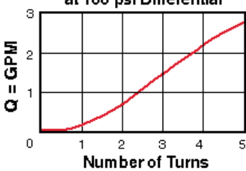
Adjustment Sensitivity at 100 psi Differential
